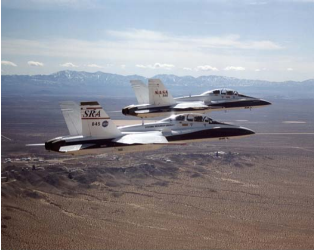
NASA Dryden Flight Research Center Photo Collection http://www.dfrc.nasa.gov/gallery/photo/index.html NASA Photo: EC01-0050-17 Date: February 21, 2001 Photo by: Lori Losey Two F/A-18B aircraft involved in the AFF program return to base in close formation with the autonomous function disengaged.
