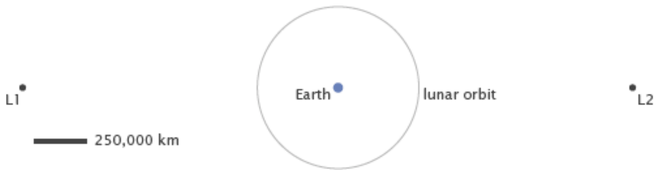
Figure 7: The L1 Lagrange point. The Lagrange point is 1.5 million kilometers away from Earth, five times farther than the moon. (NASA, 2009)
