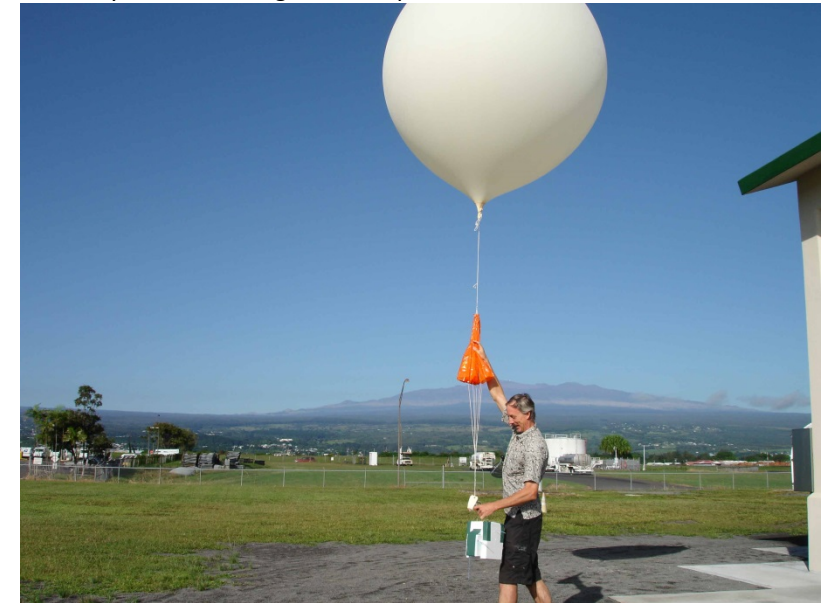
Radiosonde being launched by NOAA Earth System Research Lab
