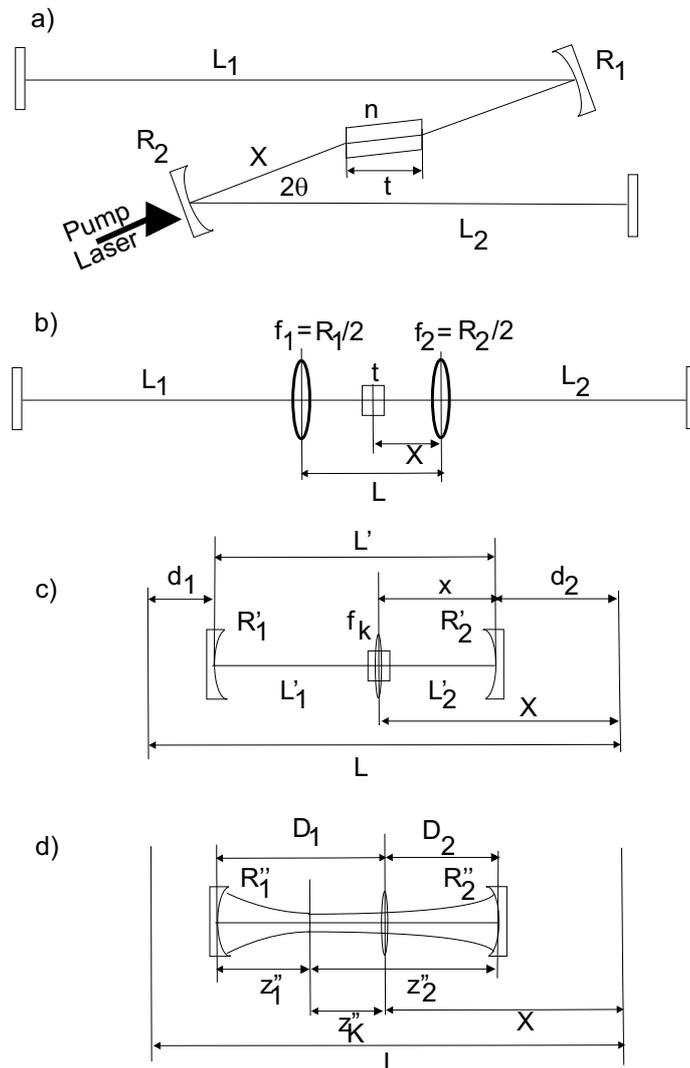
Figure 1: a) Four-mirror resonator with gain medium of thickness  $t$ . b) Equivalent resonator with lenses. c) Equivalent two-mirror resonator by imaging of the end mirrors. d) The gain medium is replaced by a Kerr-Lens in its center. The Kerr-Lens can be included in the mirrors of a new two-mirror resonator with new radii and positions from the center of the gain medium.
