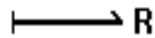
Figure 3.15: Bond graph for an ideal dissipator with sign convention and resistance causality.
