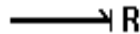
Figure 3.17: Bond graph for an ideal dissipator with sign convention and conductance causality.
