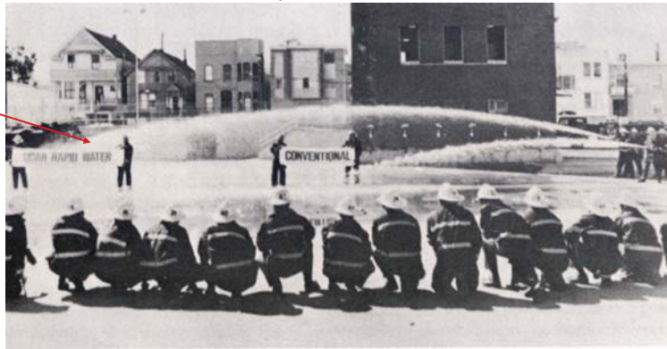
Enhancement of fire-hose range by addition of small amounts of polyethylene oxide to water. (Photograph, courtesy of Union Carbide Corporation.)
