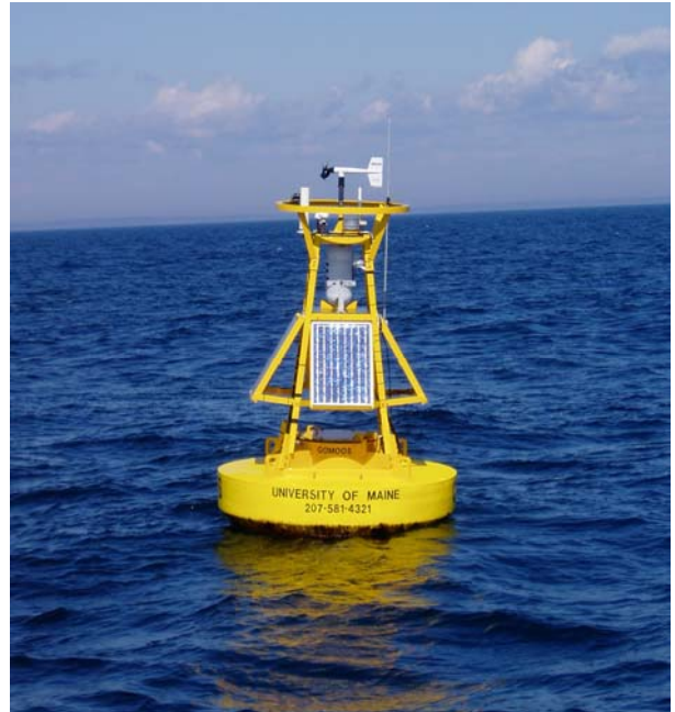
GoMOOS buoy (next version of GLOBEC buoy) has four 40 Watt solar panels and four 40 ah glass mat batteries.
