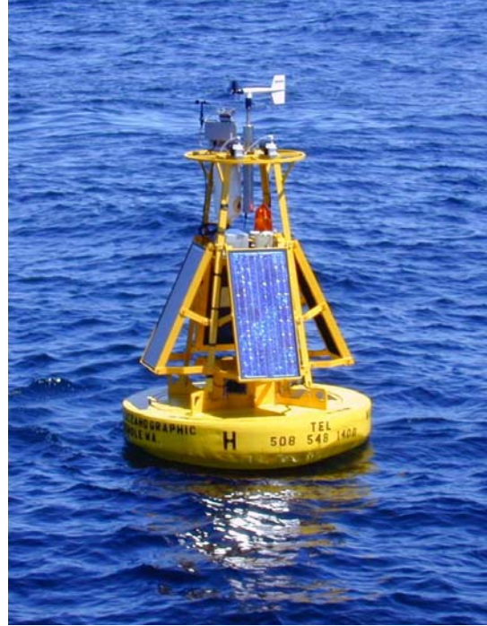
AIRMAP ozone buoy deployed in the Gulf of Maine has four 64 Watt solar panels charging four 40 ah glass mat batteries.
