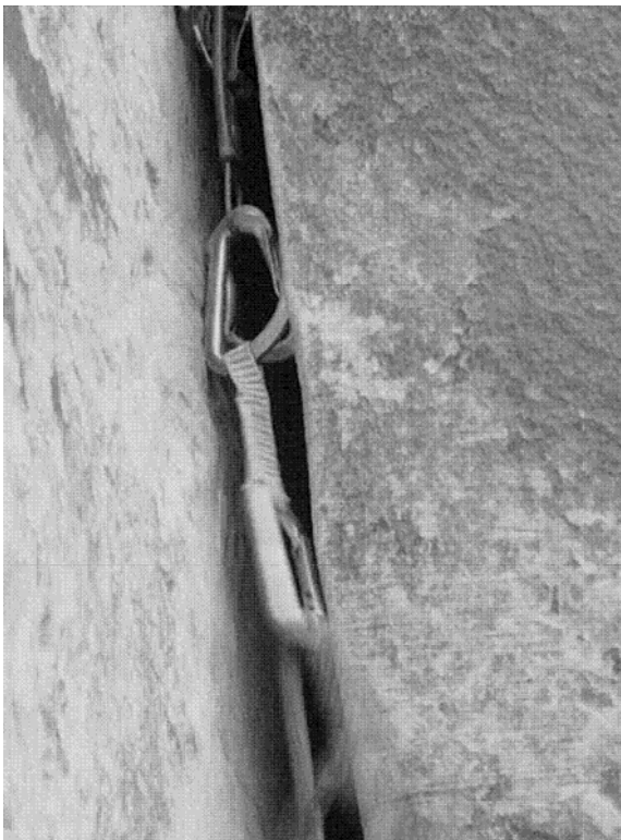
Figure 1 Video clip frame of a carabiner gate rubbing against a crack edge during a simulated fall. (stolen by my permission from an article that I wrote for the American Alpine Club)
