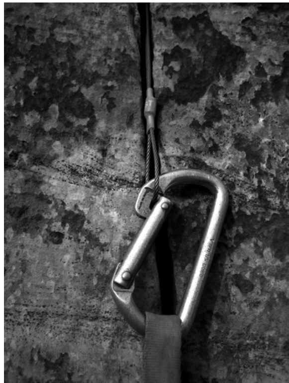
Figure 2 Carabiner gate notch caught on gear. (again, this figure is already mine, so I don't have to say that it is shamelessly stolen from myself....)
