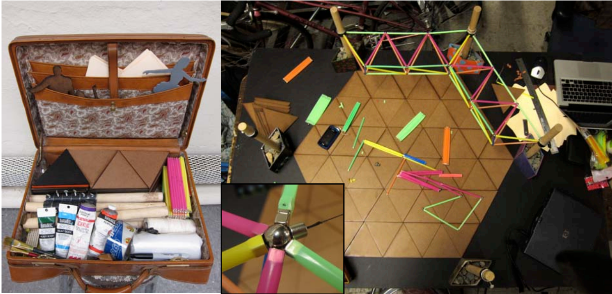
The model kit packed into a compact case, and unpacked for tinkering with structure and space. Inset detail of magnetic space frame node.
