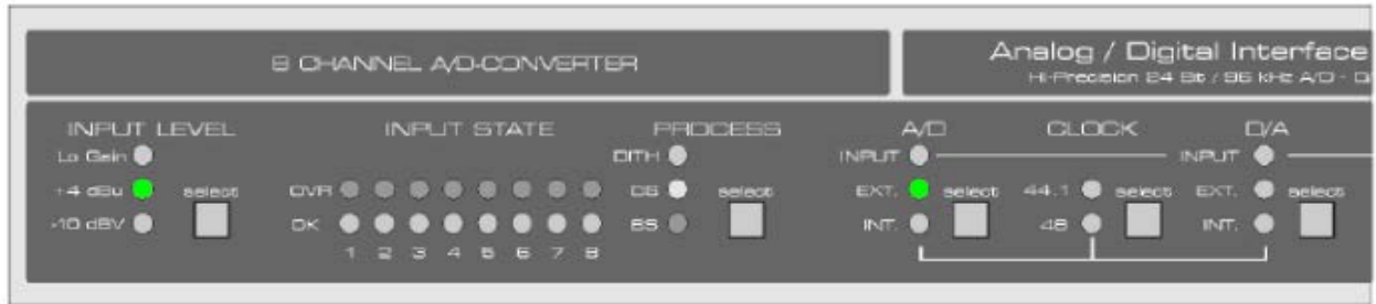
FIGURE 1. RME ADI-8 DS settings to be used for recording sessions (D/A clock settings irrelevant) (© RME Audio. With edits. All rights reserved. This content is excluded from our Creative Commons license. For more information, see http://ocw.mit.edu/help/faq-fair-use/ )
