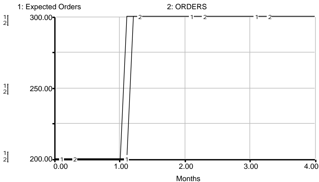
Figure 6: Behavior of the model with DT = 0.1 months and “TIME TO CHANGE EXPECTATIONS” = 0.1 months
