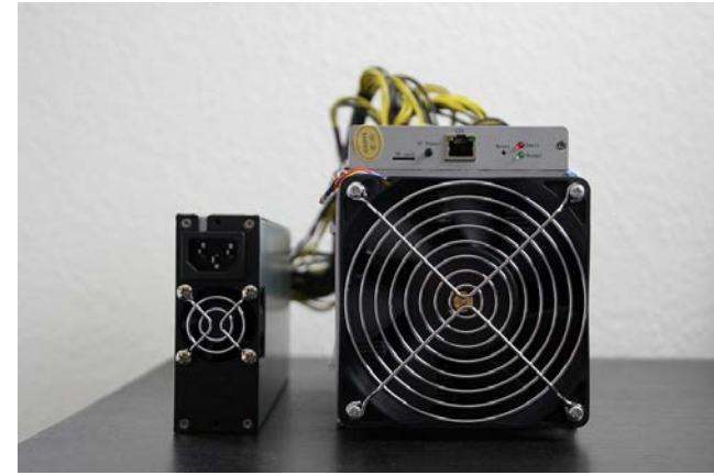
Application Specific Integrated Circuit (ASICs) 2013 – 2018 4 – 16 TH/S
