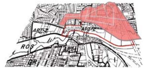
A zoning overlay is added over existing zoning to create a set of requirements that seek to protect the character of Medford Square, while unifying the east and west sides into a cohesive, vibrant, mixed-use center.
