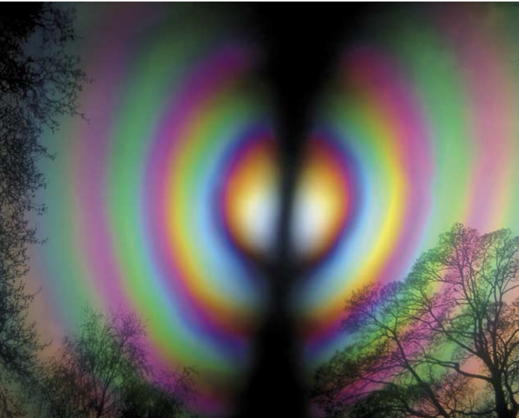
Bristol (U.K.) sky is photographed through a “black-light sandwich,” producing patterns of interference of polarized light. (From M. V. Berry, B. Handari and S. Klein, 1999, Black plastic sandwiches demonstrating biaxial anisotropy, European Journal of Physics 20:1–14.)
