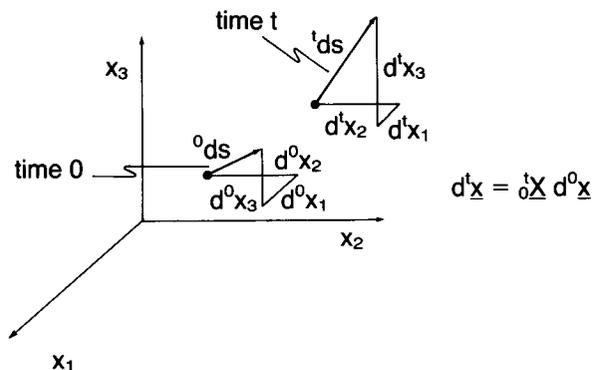
Fiber  $d^0\underline{x}$  of length  ${}^0ds$  moves to become  $d^t\underline{x}$  of length  ${}^tds$ .
